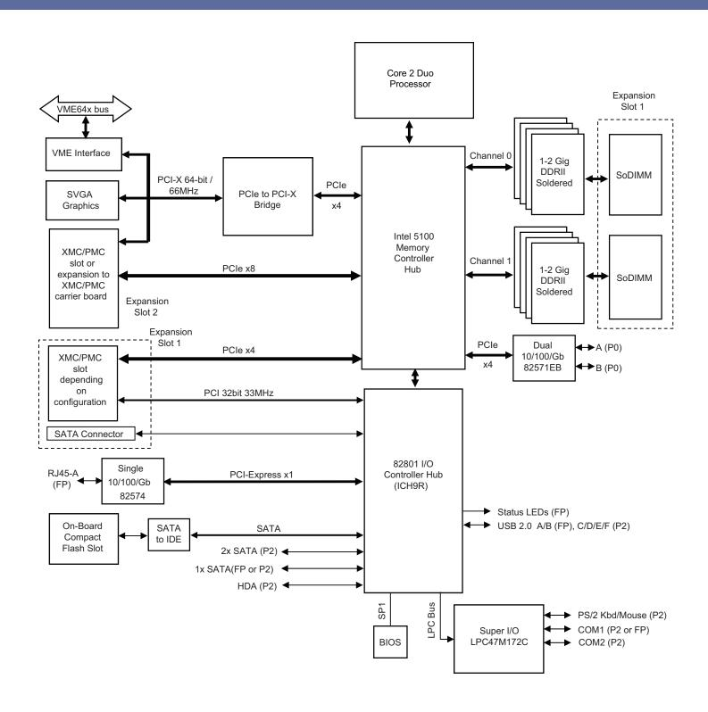
Figure 1: LV1 Block Diagram
