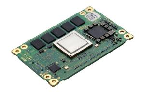
The CM10 is mechanically compliant to the COM Express Mini format. Due to the multitude of I/O offered by the ARM Cortex-A15 processor, however, the pin assignment differs from the standard COM Express type 10.
