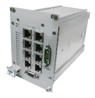
The SF1 is a stand-alone, unmanaged industrial Fast Ethernet switch that comes in a compact 3U, 18HP, 19" cassette. It provides eight channels at the front panel accessible through RJ45 connectors.
