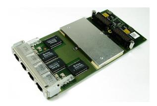
The P602 is a Gigabit Ethernet XMC mezzanine card suitable for any XMC compliant single-board computer or host carrier board in any type of bus system, i.e. CPCI, VME or on any type of stand-alone SBC. Compared to PMC, the XMC standard defines a different board-to-board connector for support of PCI Express®.
