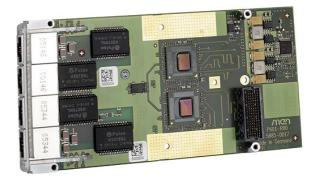
The P601 is a Gigabit Ethernet XMC mezzanine card suitable for any XMC compliant single-board computer or host carrier board in any type of bus system, i.e. CPCI, VME or on any type of stand-alone SBC. Compared to PMC, the XMC standard defines a different board-to-board connector for support of PCI Express®.
