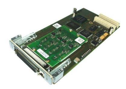
The P506 is a 32-bit/33MHz PMC with four CAN interfaces. They support CAN Protocol Version 2.0A/B, standard and extended data frames, remote frames, 0..8 bytes data length and a programmable data rate of up to 1 Mbit/s.
