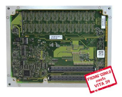
The CB70C is a member of a new family of Rugged COM Express® modules which is controlled by a third generation Intel® Core™ i7 processor running at up to 3.1 GHz maximum turbo frequency bringing state-of-the-art PC technology onto a small form factor. This means a scalable performance with 1 up to 4 cores, integrated graphics, as well as support of Intel® AMT or Open CL 1.1.
