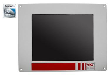
The DC2 is equipped with an internal 9 to 36 V (12 VDC nom. or 24 VDC nom.) wide-range power supply and able to operate in a -40 to +70°C environment (+85°C for 10 minutes). It complies with the EN 50155, class Tx railway standard when used with an optional includable PSU suited for railway applications. All electronic components are soldered to withstand shock and vibration and prepared for conformal coating.
