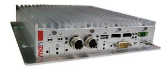
The BC1 is a maintenance-free box computer that has been designed for independent use or as display computer electronics for use in railway applications, commercial vehicles, mobile machines, avionics and mission-critical industrial control systems with visualization requirements.
