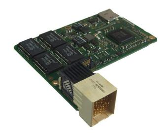
in full mesh architecture via the backplane. The GM1 is used to implement four Gigabit Ethernet interfaces which are led to the backplane via CompactPCI<sup>®</sup> Serial connector P6. All four interfaces are controlled by one Ethernet controller which supports the IEEE 802.3x standard.
