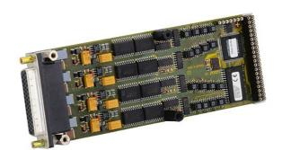
The mezzanine card M66 provides 32 binary process signals on one single M-Module, which is the largest number of binary channels ever seen on a mezzanine board. This allows a total of 128 signals with four M-Modules on a double Eurocard (i.e. in one slot of a VME or CPCI system). With its extremely high output
