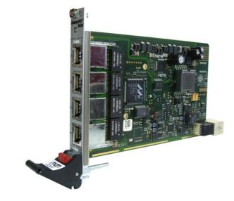
The G301 is an unmanaged 3U Ethernet switch implemented as a CompactPCI<sup>®</sup> Serial board. It occupies one peripheral slot, using a 4 HP front panel sporting 4 Gigabit Ethernet ports on RJ45 connectors. Options include M12 front connectors and a P6 connector for the rear I/O Ethernet signals from the board's fifth Gigabit Ethernet port.
