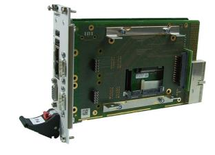
The F600 is a 4HP legacy I/O extension card for 3U Intel<sup>®</sup> based CompactPCI<sup>®</sup> single-board computers. It can be used in combination with the F14 and compatible CPU boards.
