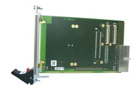
The F213 is a rugged single Eurocard CompactPCI<sup>®</sup> carrier board supporting the PMC mezzanine standard or, as an option, the Mini PCI card standard.
