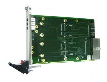
The F212U is designed for -40 to +85°C operation temperature (screened) and prepared for conformal coating in order to be used also in harsh and mobile environments.
