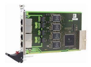
The F211 is a single Eurocard CompactPCI® networking controller that needs only one slot on the CompactPCI® bus.
