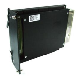
The F50C is a versatile, rugged PowerPC® based single-board computer for embedded applications with conduction cooling. It is controlled by an MPC8548, or optionally an MPC8543 PowerPC® CPU (alternatively with encryption unit) with clock frequencies between 800 MHz and 1.5 GHz. The SBC is equipped with ECC-controlled, soldered-on DDR2 RAM for data storage, with up to 16 GB of solid-state Flash disk for program storage as well as industrial FRAM and SRAM.
