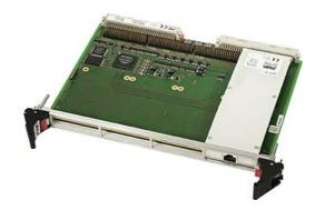
The A203N is an M-Module<sup>™</sup> carrier board for universal I/O on the VMEbus, allowing high flexibility in applications such as process and motion control, measurement and instrumentation, communication or special-purpose tasks. The M-Modules<sup>™</sup> are screwed tightly on the carrier board, and the board needs only one slot on the VMEbus.
