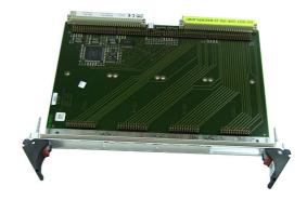
The A201S is an M-Module™ carrier board for universal I/O on the VMEbus, allowing high flexibility in applications such as process and motion control, measuring and instrumentation, communication or special-purpose tasks.
