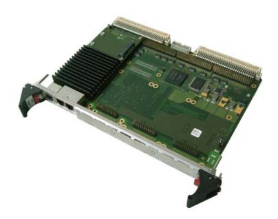
The A21B is a Freescale<sup>™</sup> QorlQ<sup>™</sup> based single-board computer for embedded industrial applications. The SBC features full VME64 support and can be used as a master or a slave in a VMEbus environment. The A21B provides 1 MB local dual-ported SRAM for slave access and communication between the local CPU and another VMEbus master.
