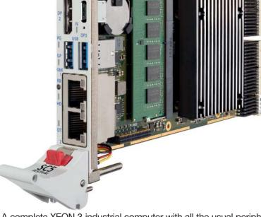
**Pic.1**: A complete XEON 3 industrial computer with all the usual peripherals on a single euroboard of 3U and with only one slot space requirement (4HP).
