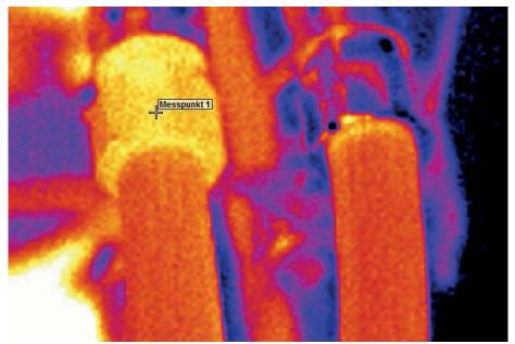
**Pic.5:** In the thermographic image, the temperature difference in the cooling tubes between primary and secondary heat exchangers can be seen very clearly
