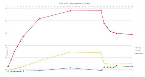
**Pic.3:** Temperature inside the rack at several measurement points. T=0 Starting system w/o CoolConduct. At T=30 starting of the coolant pump. At T=35 stable conditions.
