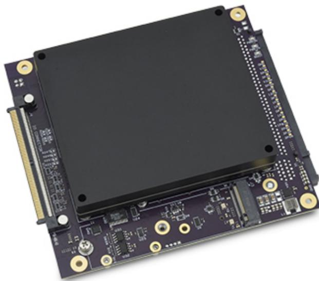
**Osbourne with AGX Orin module installed**
