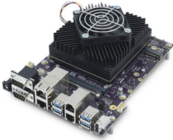
**Osbourne full kit with Orin module, fan sink, and commercial I/O adapter**
