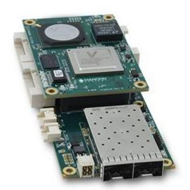
EPS-12002L switch end view, cooling solution removed
